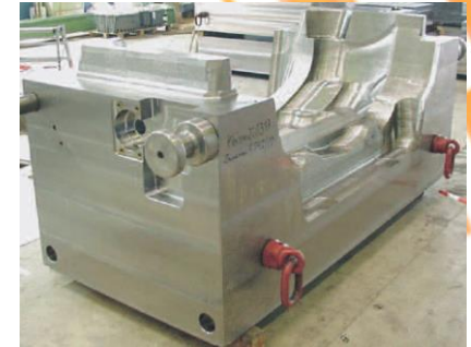
Car Bumper Mold (1160 x 1010 x 2700 mm, weight 22 metric tons)
