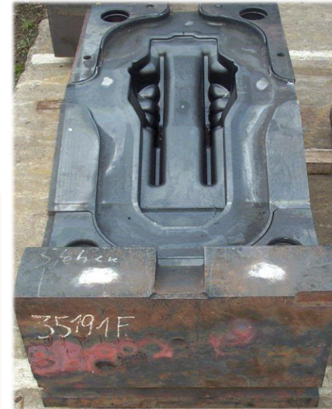
2714 ISO-B MOD large Press-Die for Aluminum-Forging, Dimensions: 965 x 620 x 1970 mm
