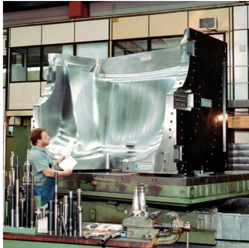
Cavity for Truck Motor Hood
