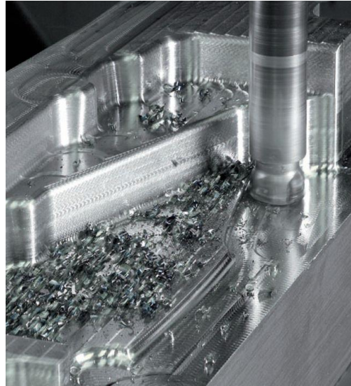
Core Part made of 2312 undergoing rough machining
