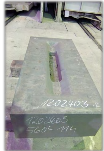
Dies after Contour-Hardening
