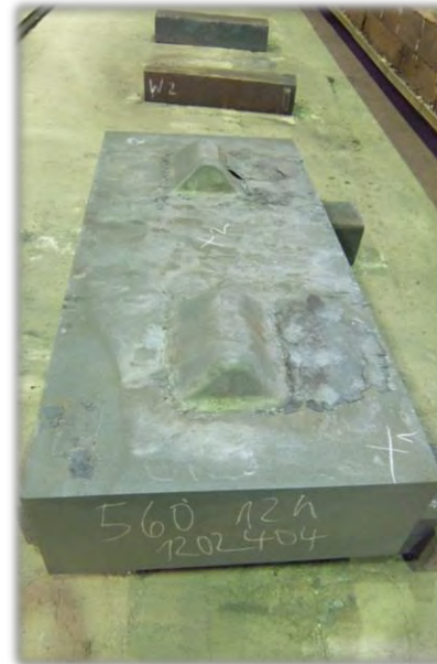
Dies after Contour-Hardening
