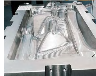
Pre-machined Mudguard Mold, prepared for Quench + Temper in Near-Net Shape (generally recommended for Standard-Grade 2711 ISO-B)
