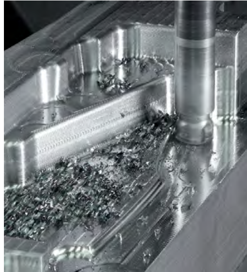
Core Part made of 2312 undergoing rough machining
