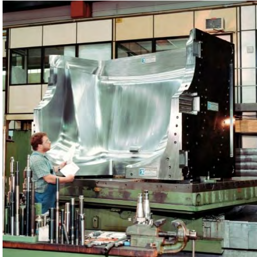
Cavity for Truck Motor Hood
