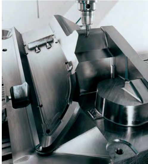
Contour milling to 3D-data
