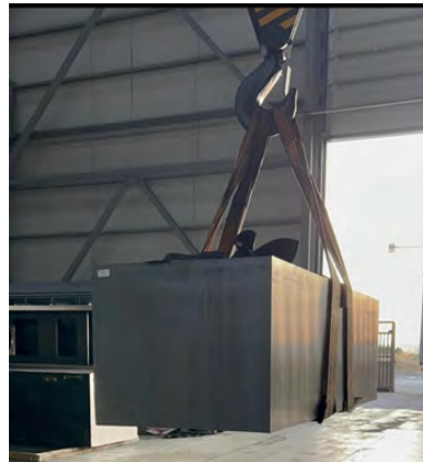
Plastic mold steel for our customer producing white goods 960x1100x3300 1.2312
